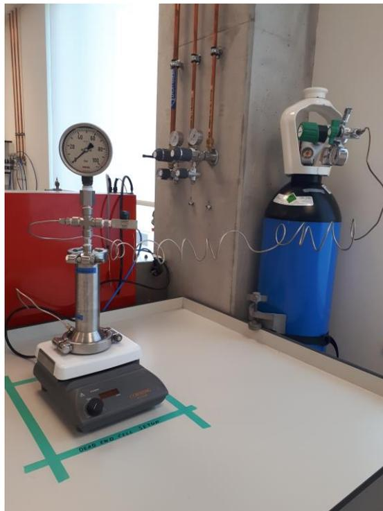
Figure 16 Figure of the dead-end RO cell setup
