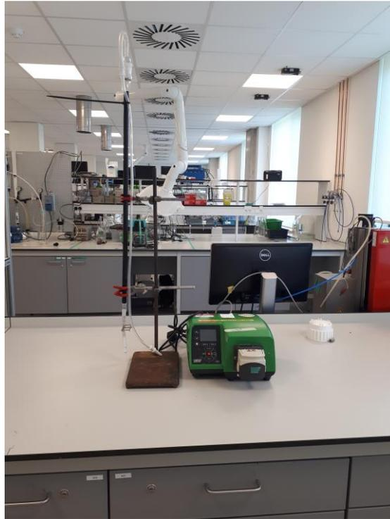
Figure 19 Figure of the single column setup
