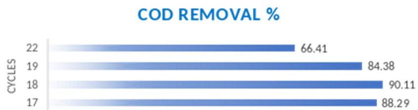
Figure 17— Laboratory study of SBR and COD (key contaminant) removal for case study 2 under different process conditions. (figure extracted from AquaSPICE 2023 General Assembly meeting presentation)
