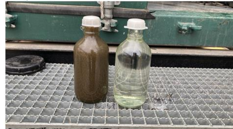
UF is operated, uf inlet and outlet shown below.
