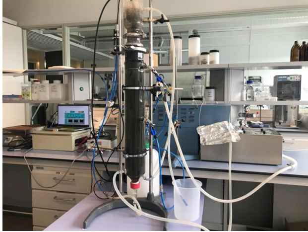
GRANULAR BIOLOGICAL REACTOR
