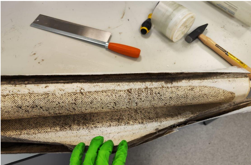
Figure 25 Membrane autopsy after the CCRO tests
