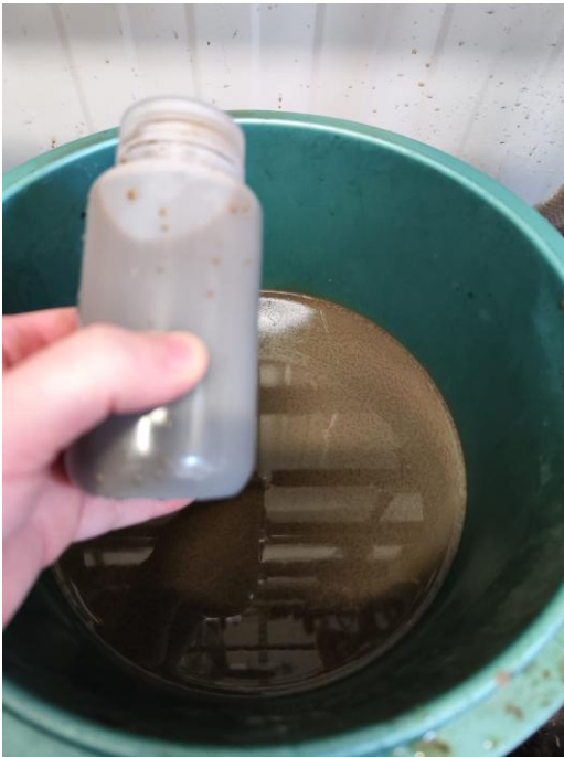
Figure 24 A sample of the water during and air flush scouring
