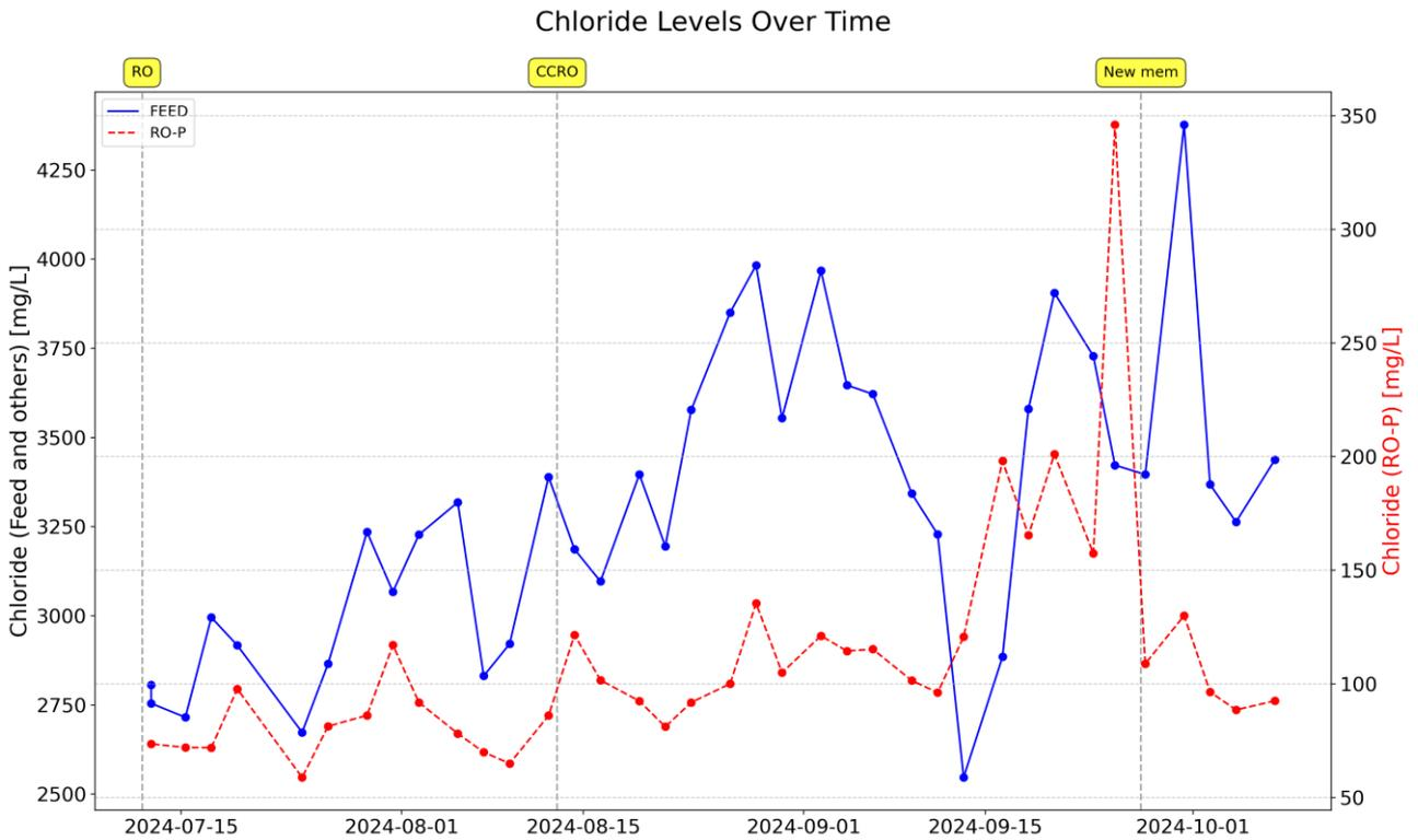
Figure 38 Chloride levels in the feed and the RO permeate
