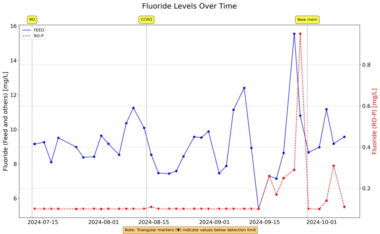
Figure 39 Fluoride levels in the feed and the RO permeate
