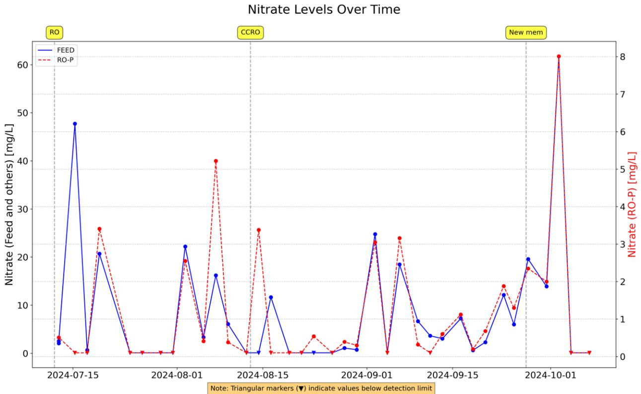
Figure 28 Nitrate levels in the feed and the RO permeate
