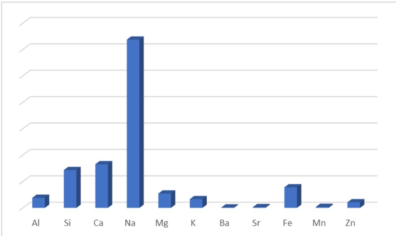
Figure 25 Relative concentrations in the ICP-OES analysis after microwave digestion. Numbers are not given as they are meaningless in a relative concentration context.
