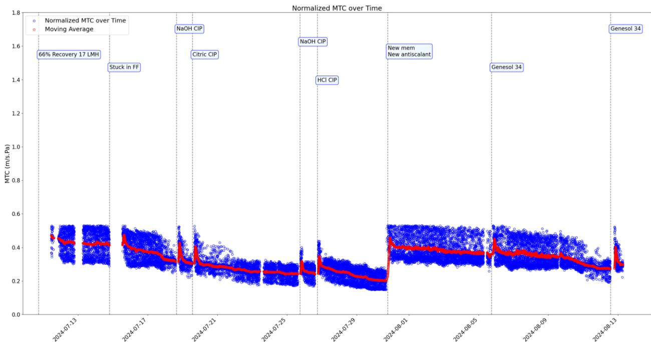
Figure 16 Membrane MTC for the RO membrane without the concentration polarization taken into account
