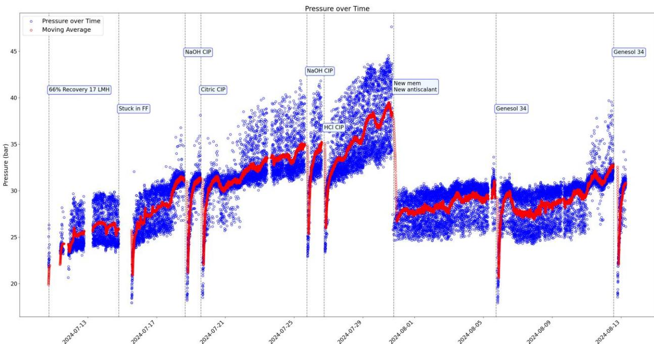
Figure 15 Average feed side pressure of the reverse osmosis
