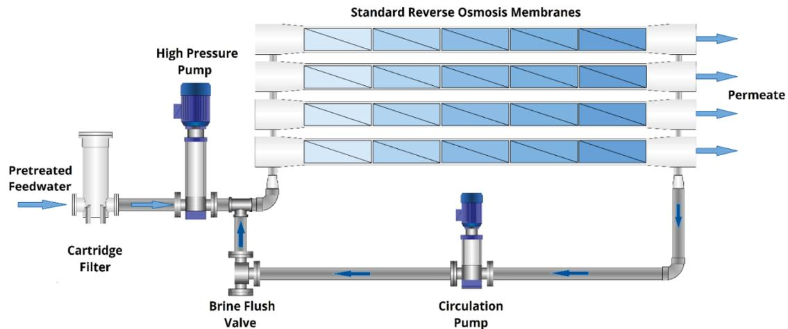
Figure 2 Schematic overview of the working principle of CCRO during closed circuit mode; after each filtration cycle the brine flush valve will open for certain amount of time [5]
