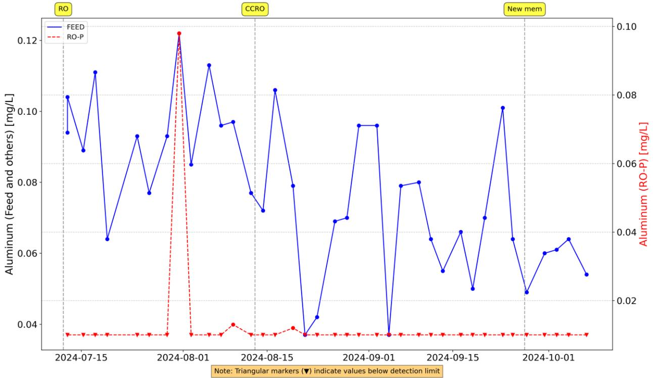
Figure 35 Aluminum levels in the feed and the RO permeate
