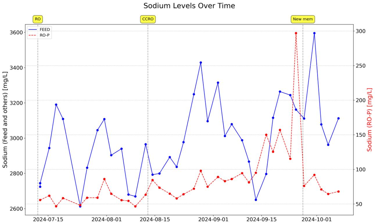
Figure 52 Sodium levels in the feed and the RO permeate
