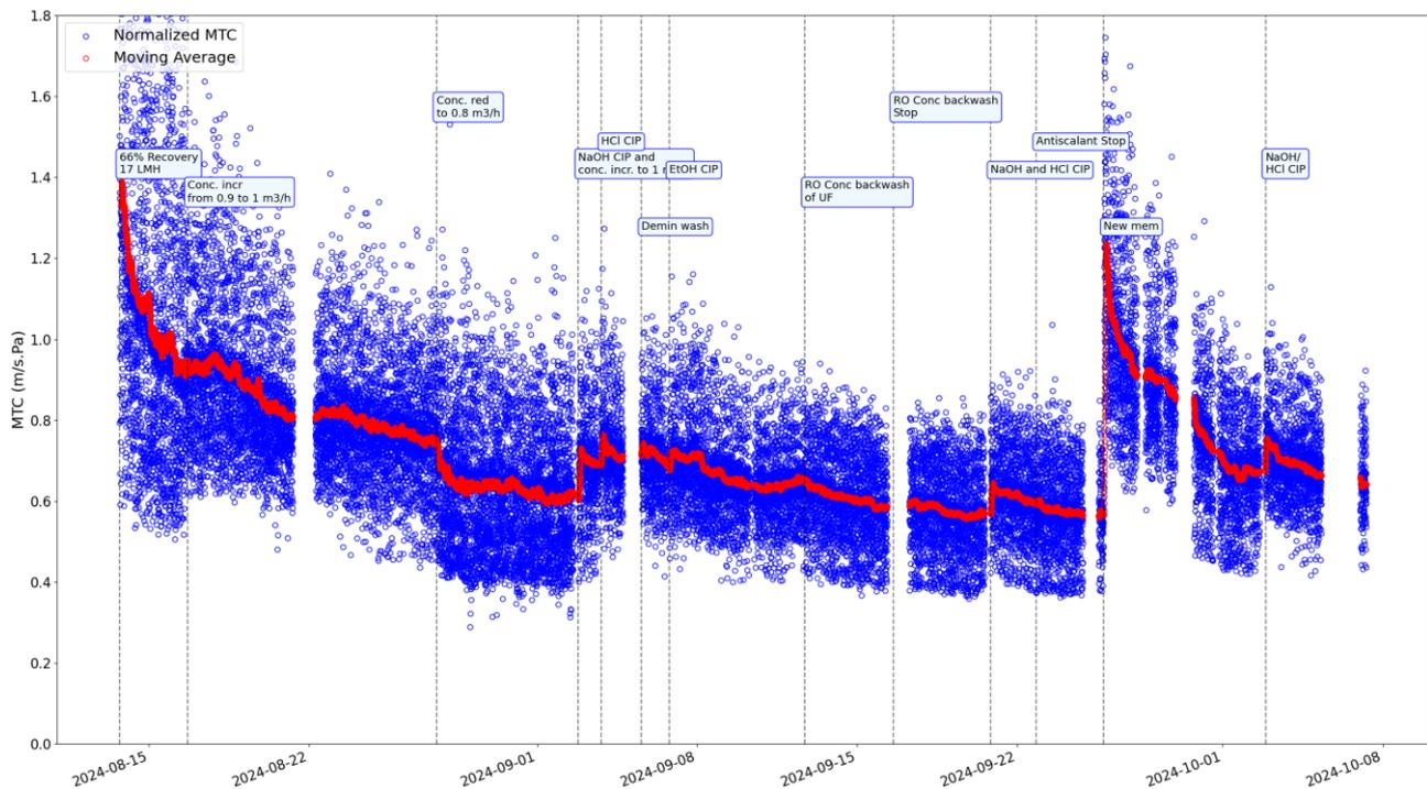
Figure 17 Membrane MTC of the CCRO
