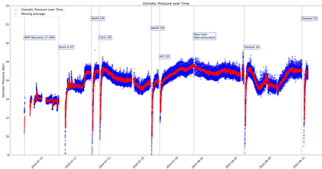
Figure 14 Average osmotic pressure of the feed and concentrate in the RO
