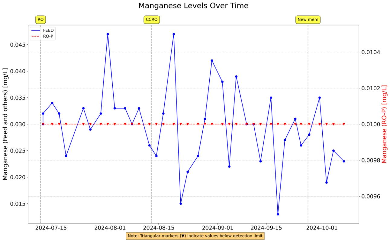
Figure 51 Manganese levels in the feed and the RO permeate
