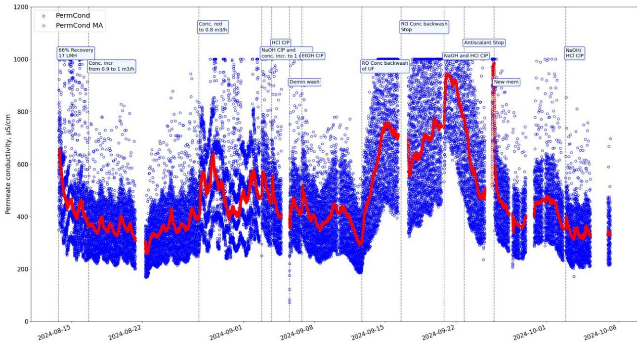
Figure 18 Permeate conductivity in CCRO mode
