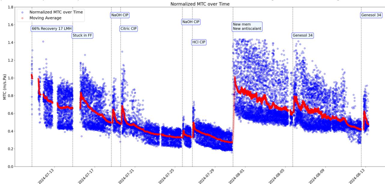
Figure 8 Normalized membrane mass transfer coefficient (MTC for the RO)
