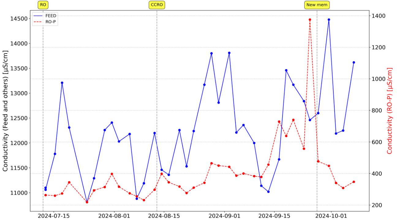
Figure 47 Conductivity of the feed and the RO permeate (Measured in grab samples in the lab)
