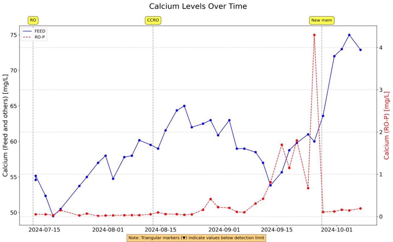
Figure 43 Calcium levels in the feed and the RO permeate
