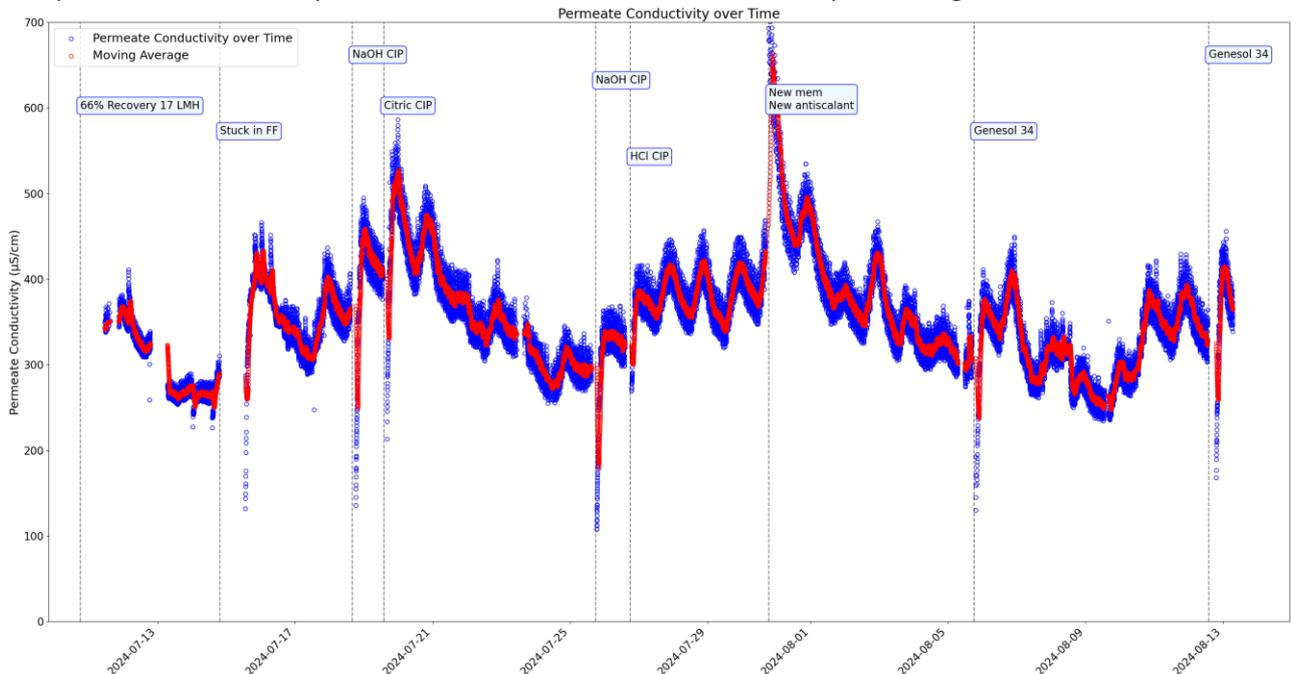
Figure 10 Permeate conductivity in RO mode
