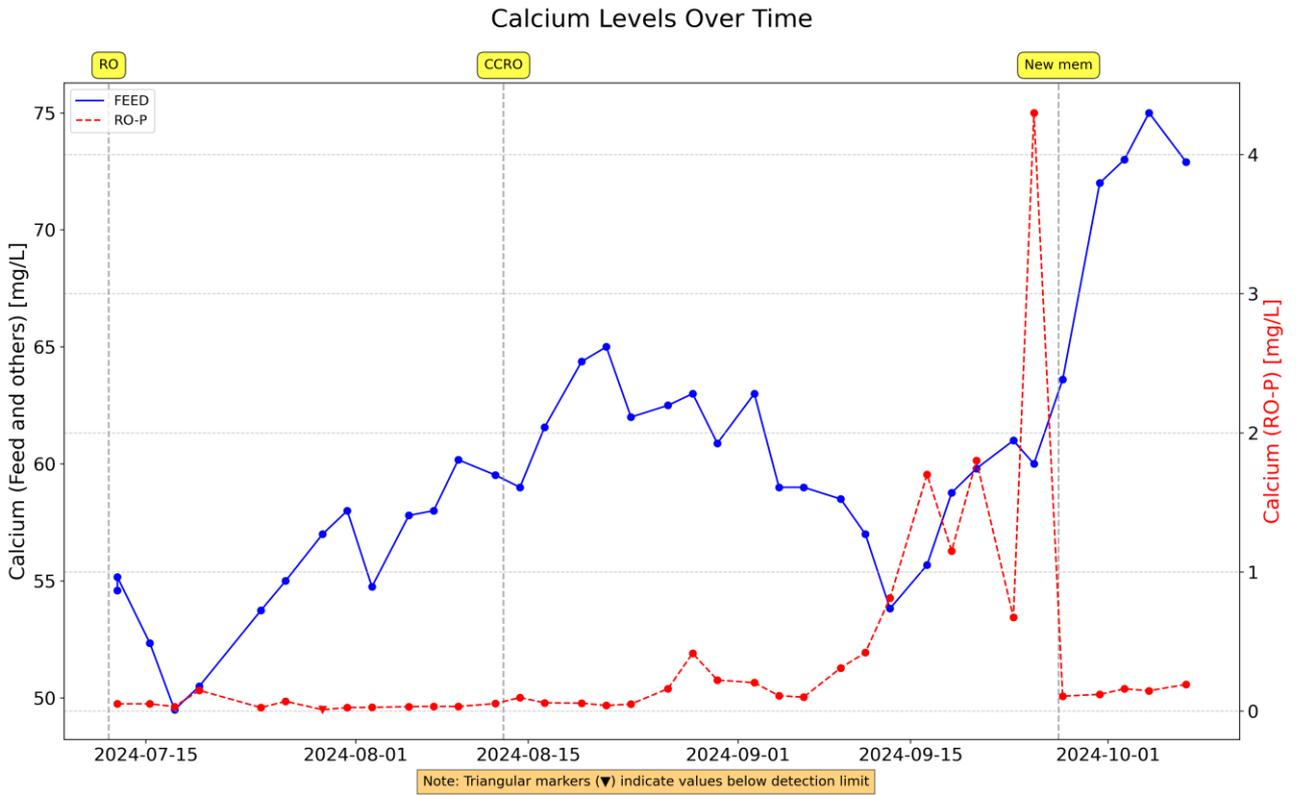
Figure 37 Calcium levels in the feed and the RO permeate
