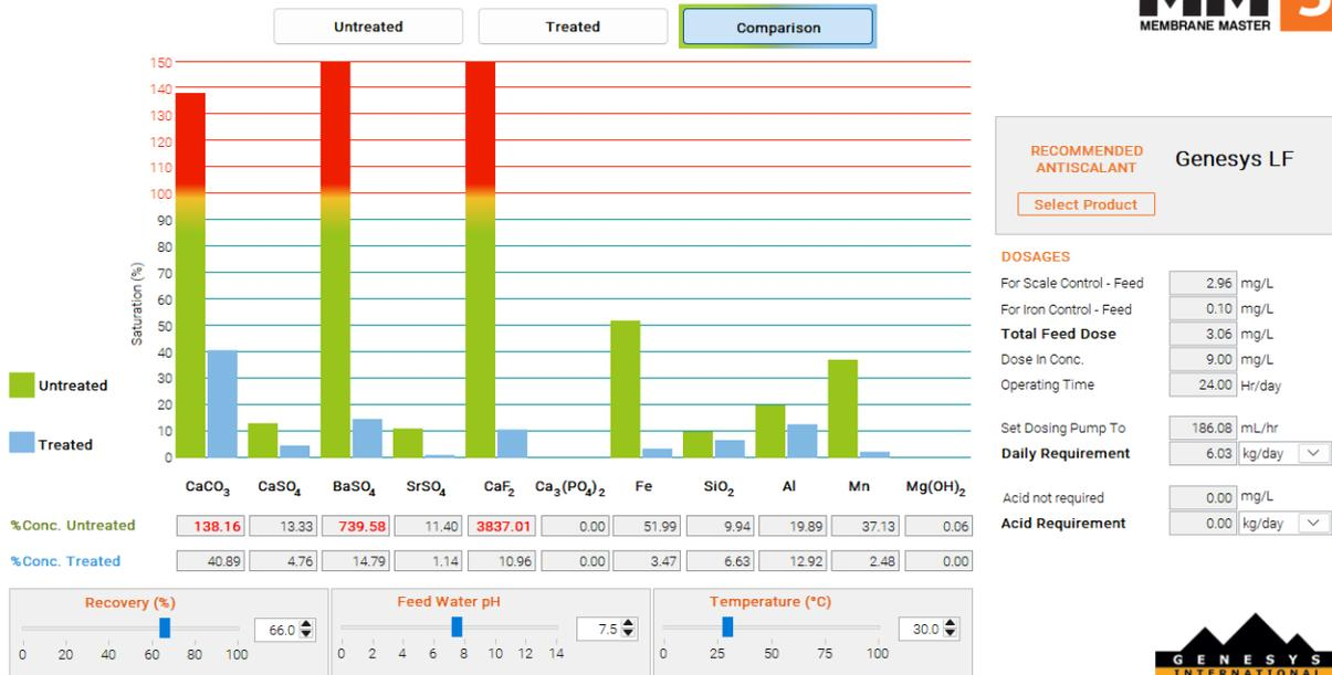
Figure 24 Scaling prediction from the Membrane Master 5 software
