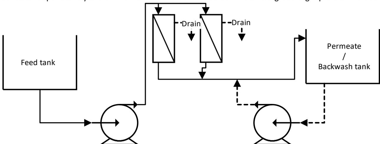
Figure 4 Simplified schematics of the UF skid
