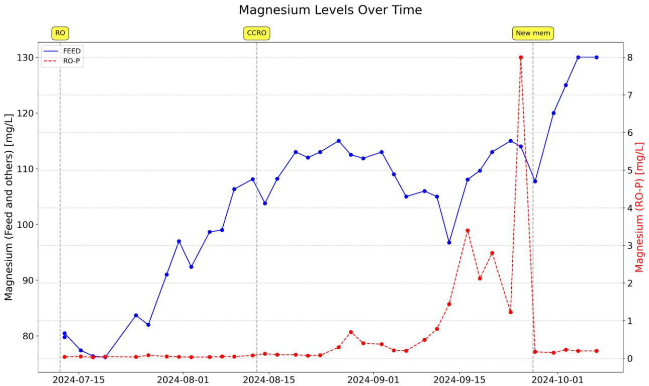
Figure 50 Magnesium levels in the feed and the RO permeate
