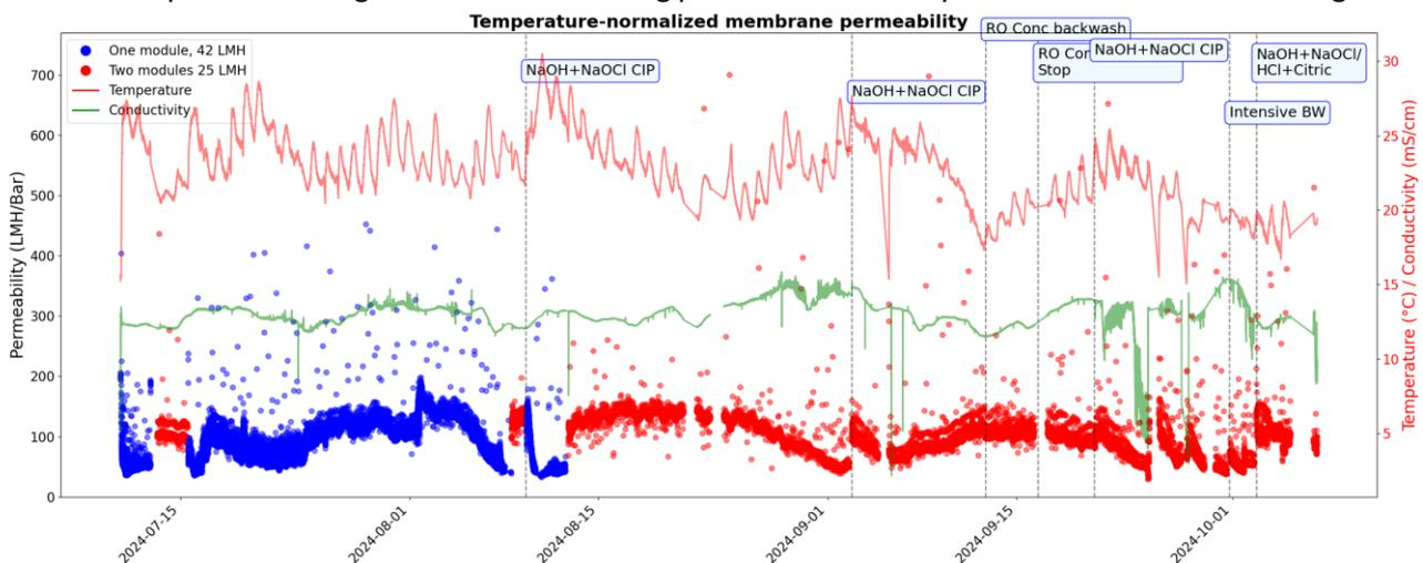
Figure 5 Temperature, Conductivity and normalized permeability of the UF in the testing period
