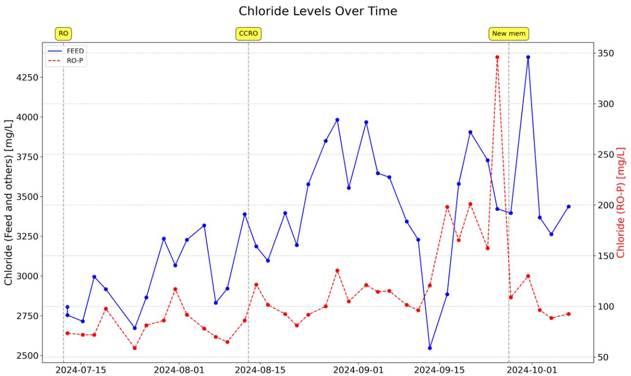
Figure 44 Chloride levels in the feed and the RO permeate
