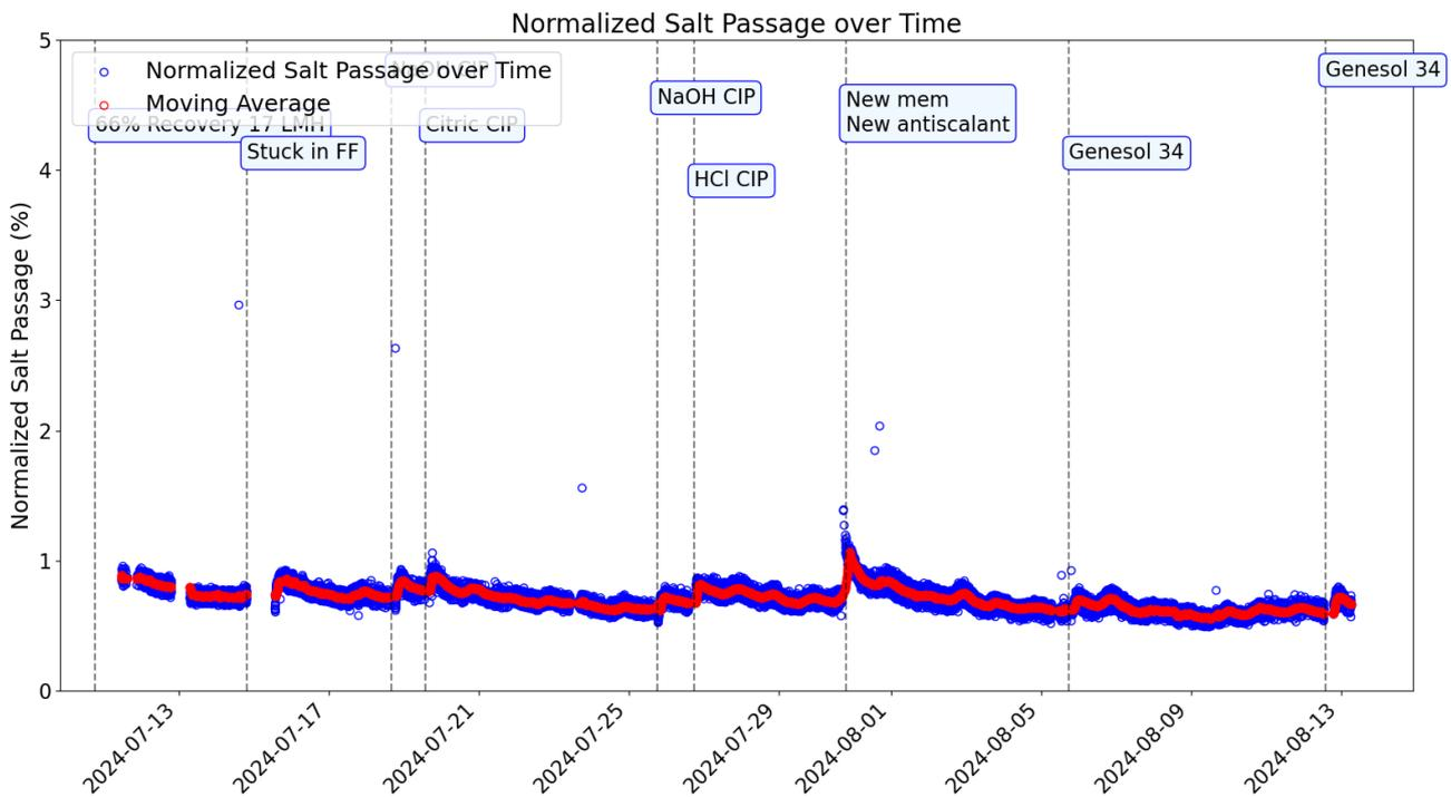
Figure 11 Normalized salt passage in RO mode
