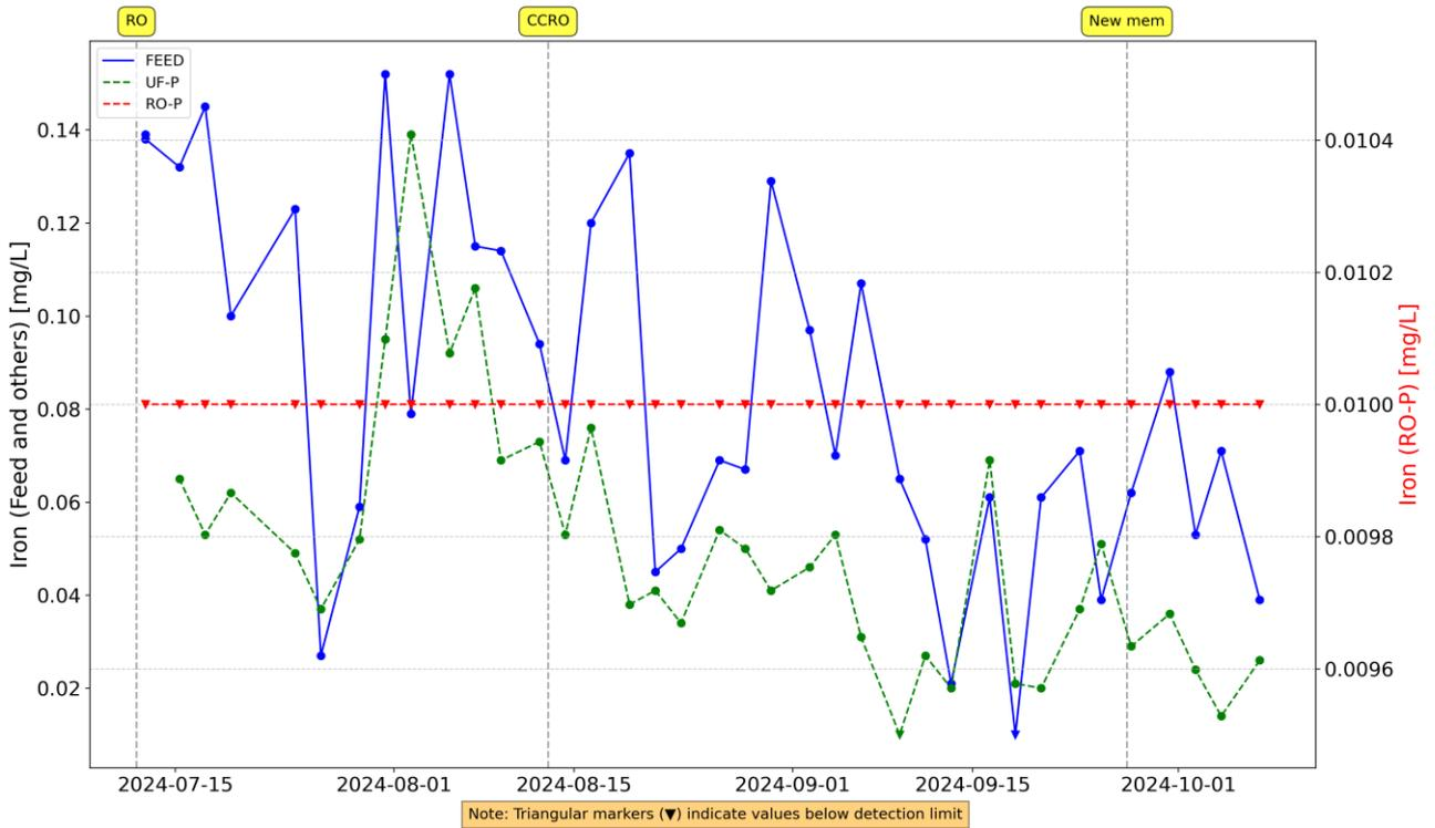
Figure 48 Iron levels in the feed and the RO permeate
