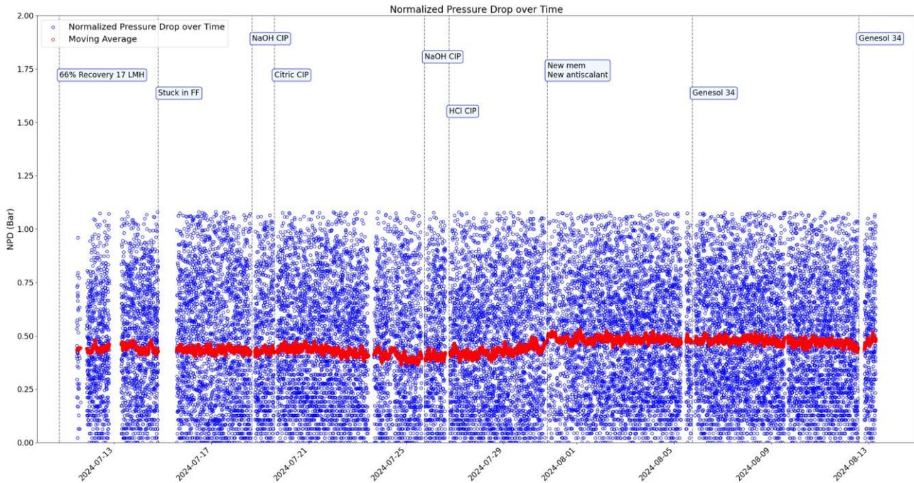
Figure 9 Feed channel pressure drop during the RO tests
