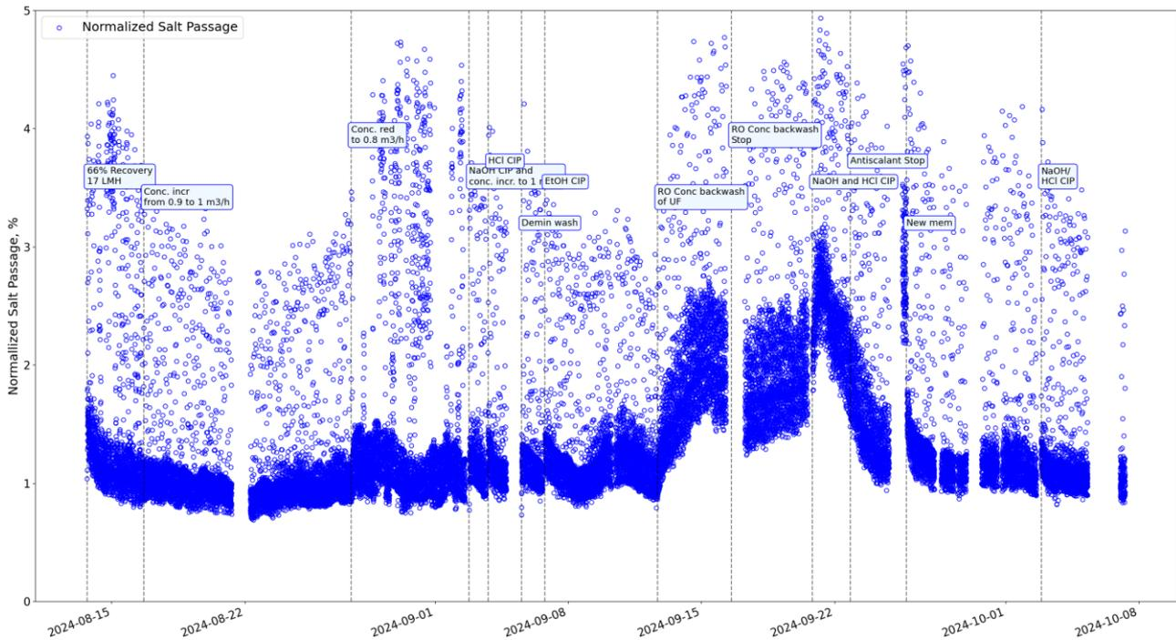
Figure 19 Normalized salt passage in CCRO mode
