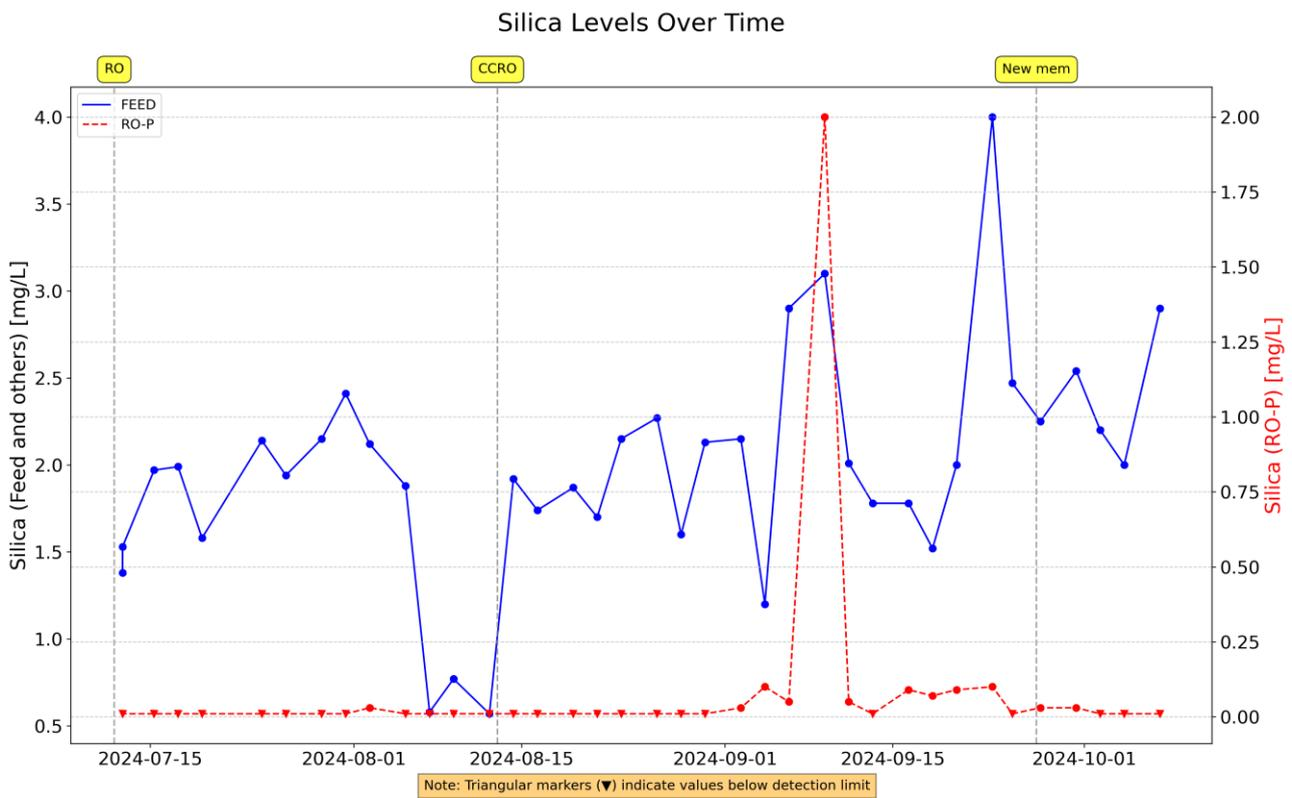
Figure 30 Silica levels in the feed and RO the permeate
