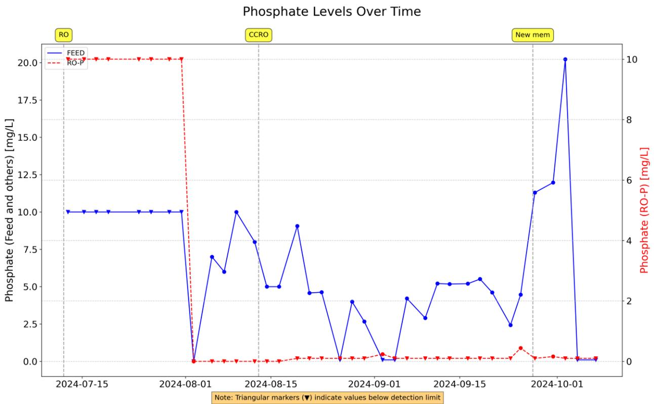
Figure 46 Phosphate levels in the feed and the RO permeate. Please note the higher detection limit in the beginning of the tests
