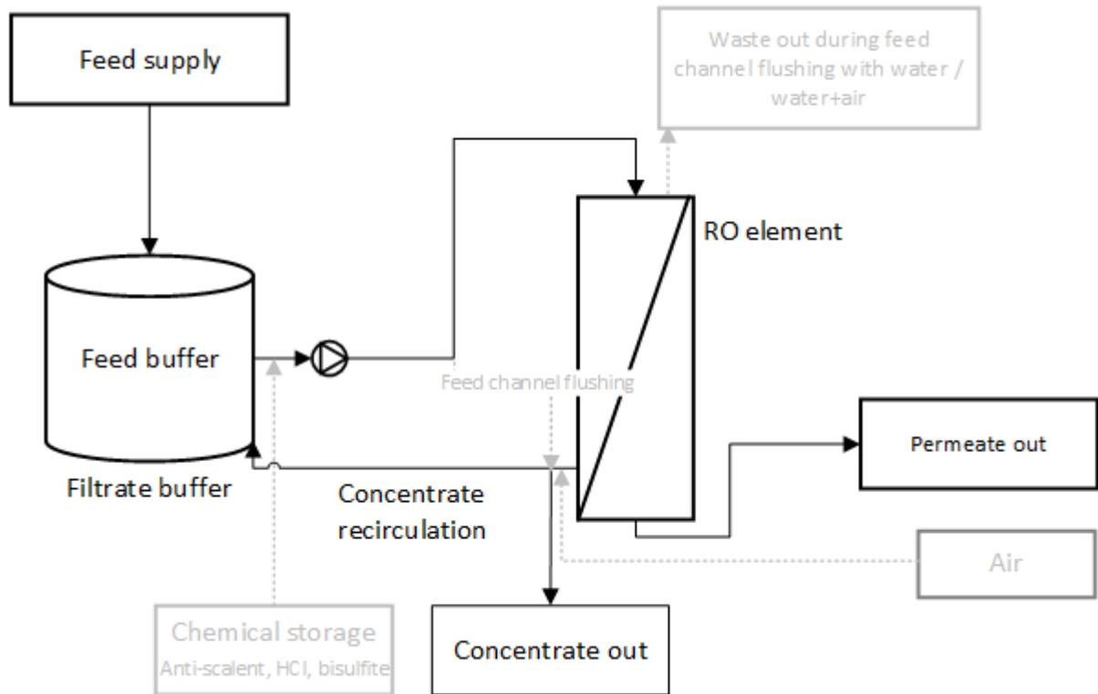
Figure 3 Schematic overview of the conventional RO module. The lines in gray are used only during cleaning in place or injection of air.
