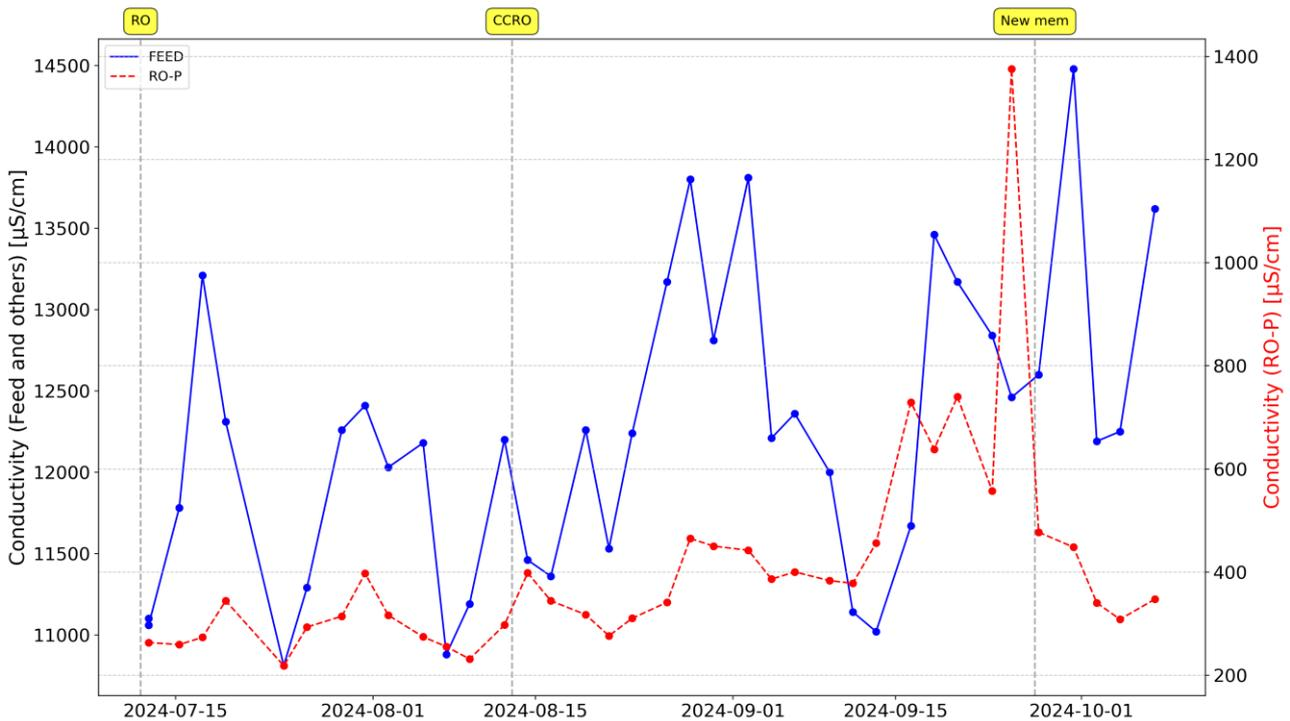
Figure 34 Conductivity of the feed and the RO permeate
