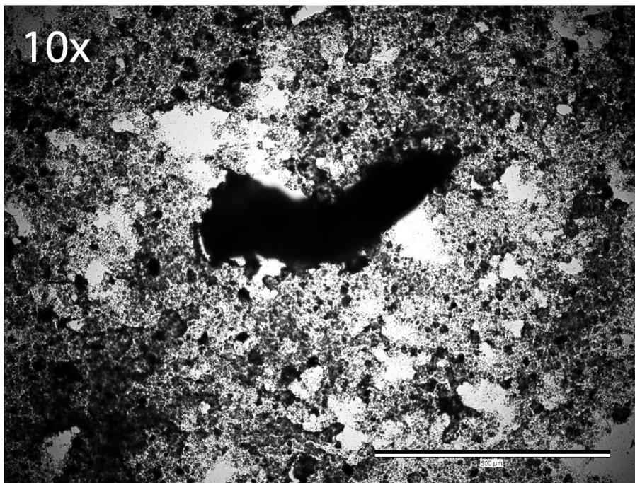
Figure 27 Optical microscopy of the fouling scraped from the membrane
