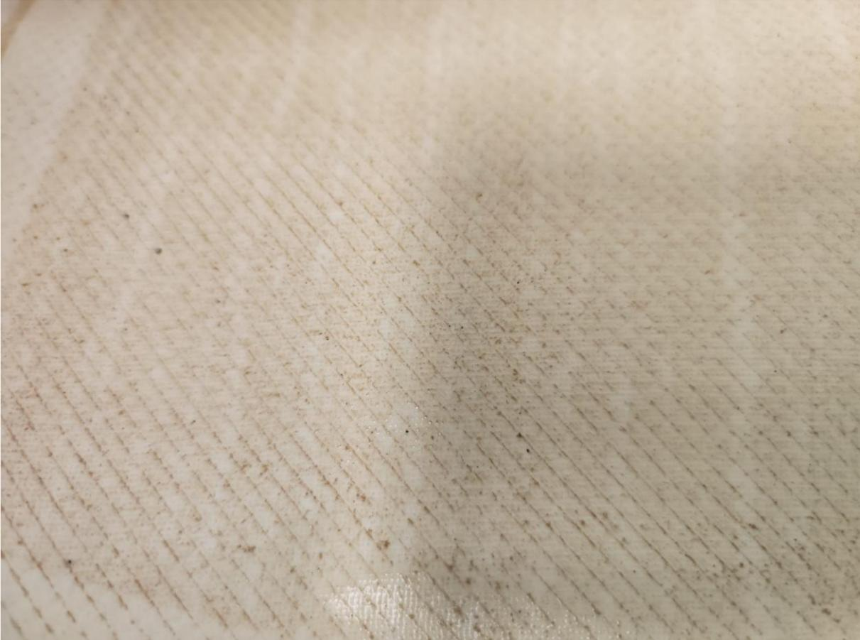
*Figure 23 Membrane autopsy on 01/08. Operation in RO mode*
