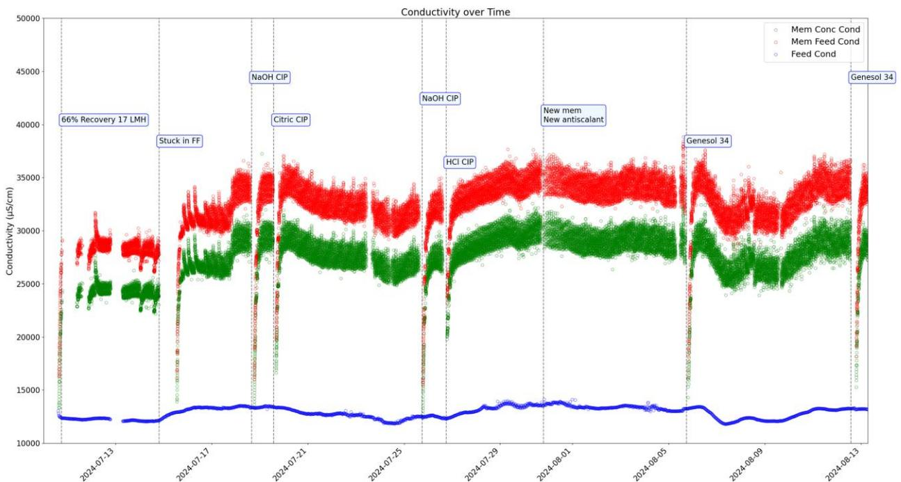
Figure 13 Conductivity on the feed and concentrate sides of the RO membrane as well as the feed conductivity.
