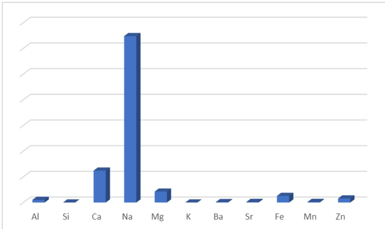
Figure 26 Relative concentrations in the ICP-OES analysis after soaking the membrane for over 1h in HCl followed by microwave digestion. Numbers are not given as they are meaningless in a relative concentration context.
