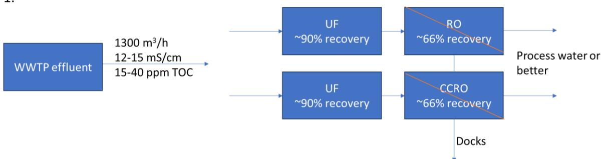
Figure 1 Schematic representation of the technologies tested at the WWTP of BASF Antwerpen
