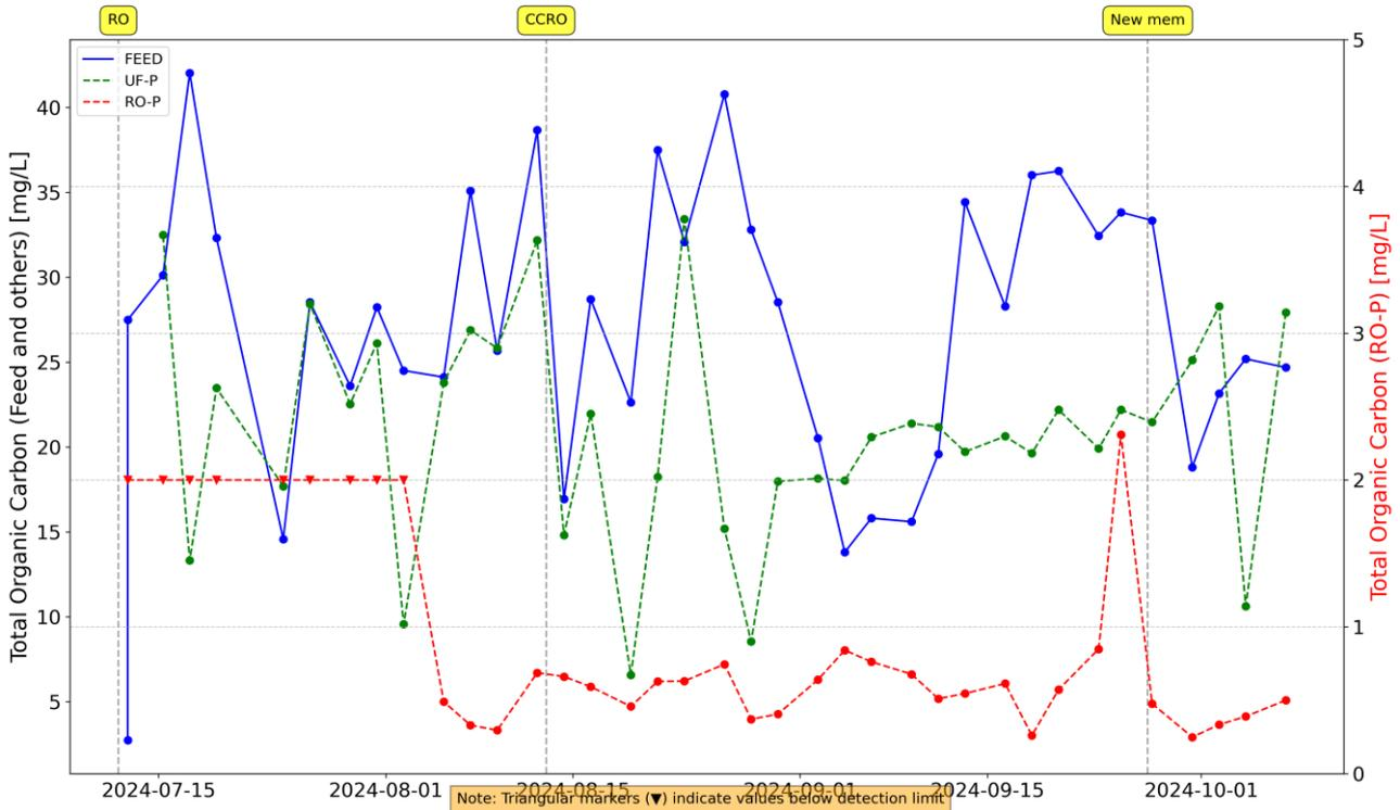
Figure 33 TOC levels in the feed and the RO permeate. Please note the higher detection limit in the beginning of the tests
