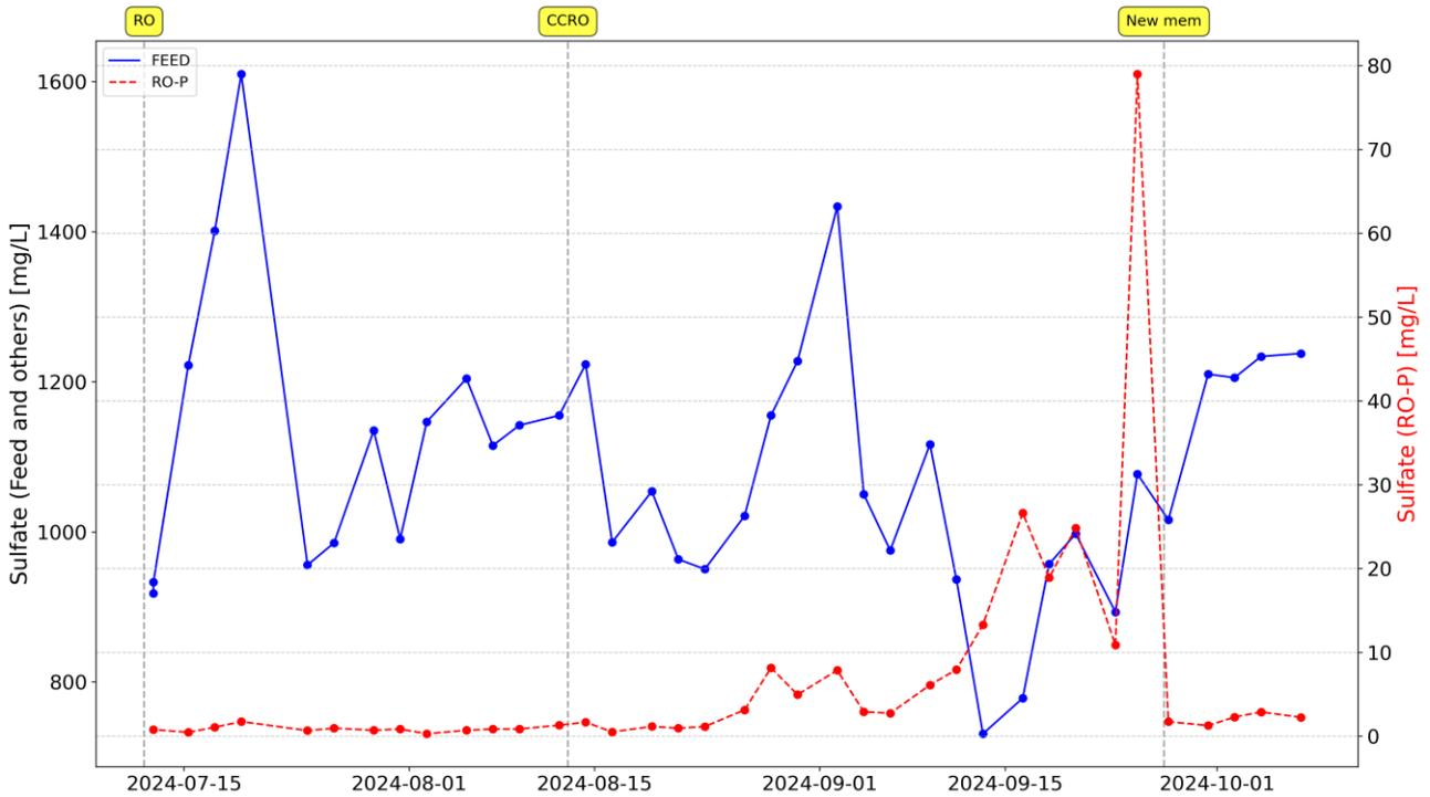
Figure 32 Sulfate levels in the feed and the RO permeate
