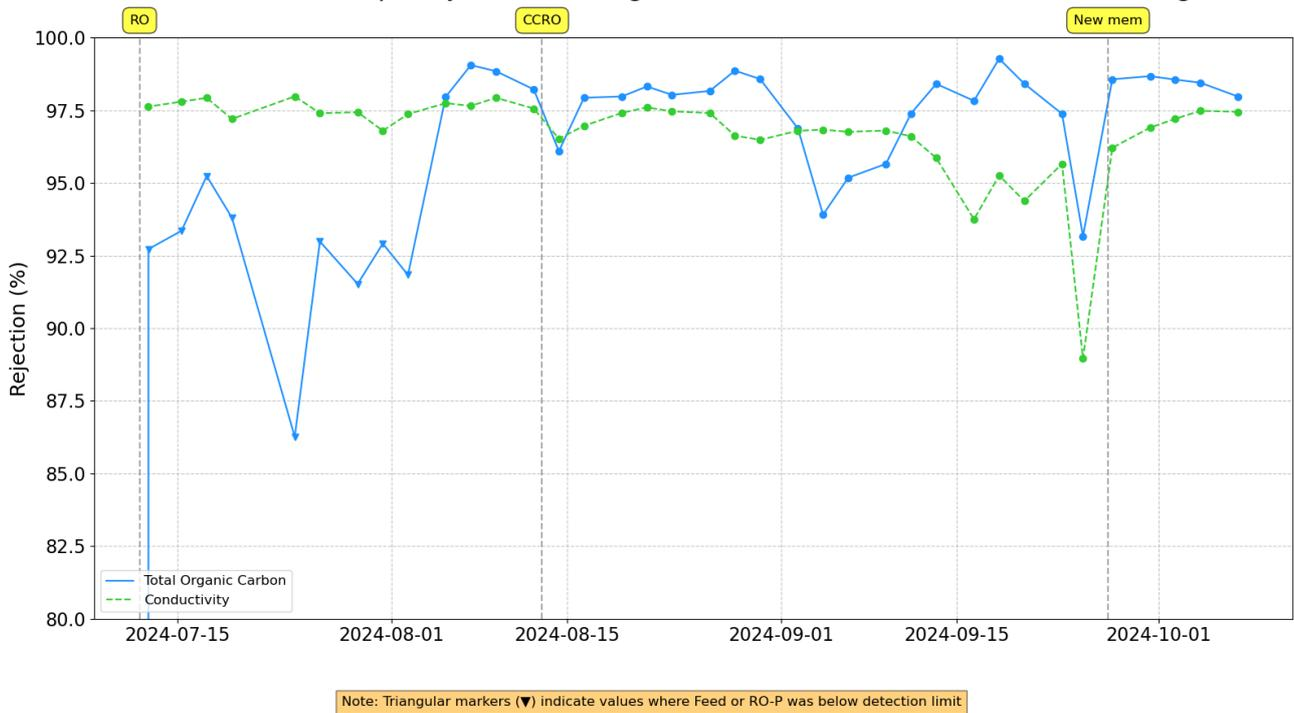
Figure 22 Rejection of conductivity and TOC during the trials for RO and CCRO
